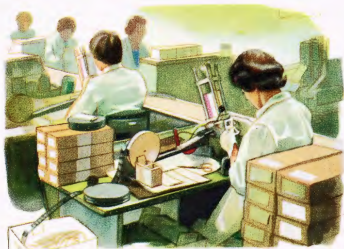
Colour transparencies are also handled at Ilford's Basildon Laboratories. They are here being fed into an automatic mounting machine
